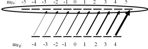
FIG. 7: Illustration of the transformation of bright to dark resonance at the  $F_g = 4 \rightarrow F_e = 5$  transition, in case of depolarizing  $F_e = 5$  level collisions between Cs and buffer gas atoms.
