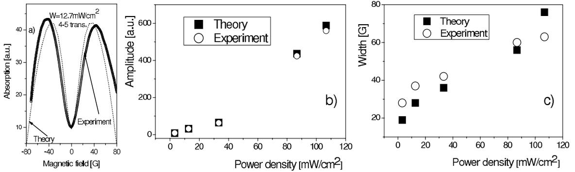
FIG. 10: Comparison between theory and experiment, for  $F_g = 4 \rightarrow F_e = 5$  transition and excitation by circularly polarized light: (a) - magneto-optical resonance experimental and theoretical profiles; (b) - magneto-optical resonance amplitude as a function of the light power density; (c) - magneto-optical resonance width as a function of power density.
