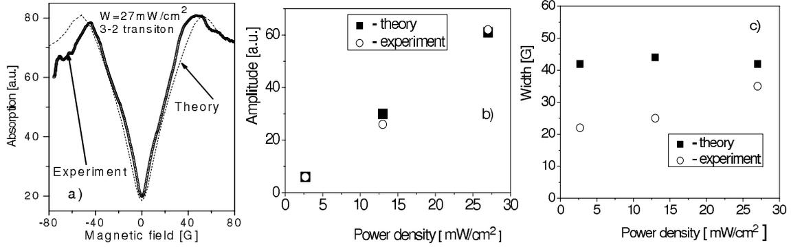
FIG. 8: Comparison between theory and experiment, for  $F_g = 3 \rightarrow F_e = 2$  transition and excitation by linearly polarized light: (a) - magneto-optical resonance experimental and theoretical profiles; (b) - magneto-optical resonance amplitude as function of the light power density; (c) - magneto-optical resonance width as a function of power density.
