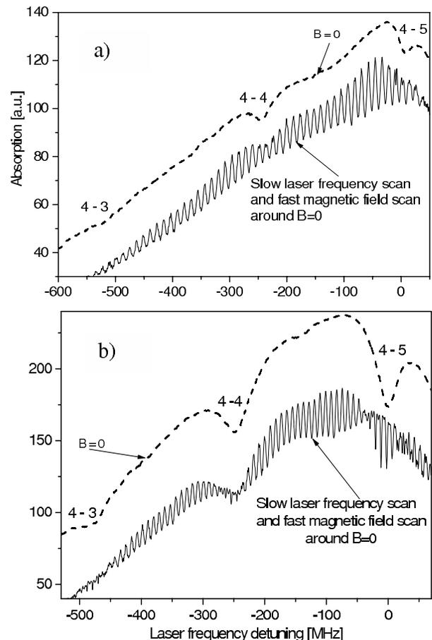
FIG. 5: Magneto-optical resonances superimposed on the ETC absorption spectrum (solid line) and the corresponding part of the ETC absorption spectrum (dashed line) at the  $F_g = 4$  absorption line for two different laser powers  $W=13\text{mW}/\text{cm}^2$  (a) and  $W=133\text{mW}/\text{cm}^2$  (b). Cs source temperature is  $131^\circ\text{C}$ ,  $L = \lambda$ , linearly polarized laser light.
