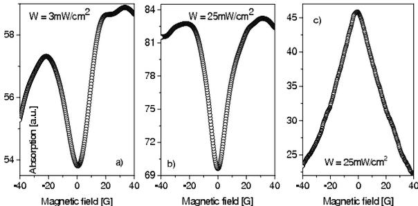
FIG. 6: Illustration of dark magneto-optical resonances observed at  $F_g = 3 \rightarrow F_e = 2$  (a) and  $F_g = 3 \rightarrow F_e = 4$  (b) transitions for slow atoms, and non-coherent feature (c) observed for fast atoms. Cs source temperature is  $112^\circ\text{C}$  and  $L = \lambda$ .
