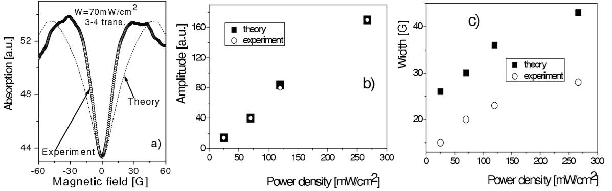
FIG. 9: Comparison between theory and experiment, for  $F_g = 3 \rightarrow F_e = 4$  transition and excitation by linearly polarized light: (a) - magneto-optical resonance experimental and theoretical profiles; (b) - magneto-optical resonance amplitude as a function of the light power density; (c) - magneto-optical resonance width as a function of power density.
