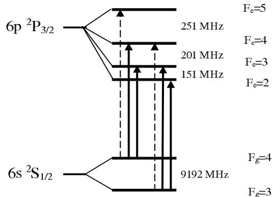
FIG. 1: Energy-level diagram for the  $D_2$  line of  $^{133}\text{Cs}$ .  $F_g \rightarrow F_e \leq F_g$  transitions (solid line) are distinguished from  $F_g \rightarrow F_e > F_g$  transitions (dashed line).
